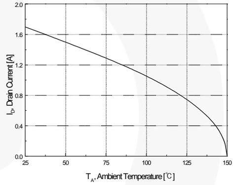
**Figure 10. Maximum Drain Current vs. Ambient Temperature**
