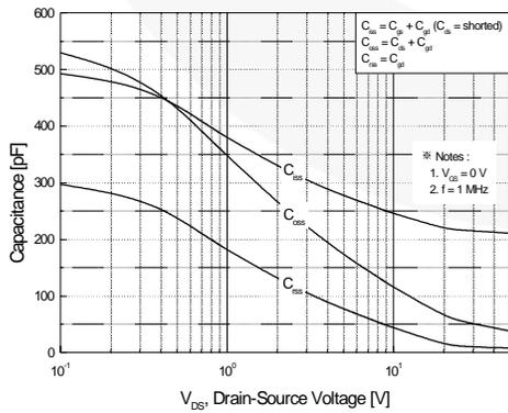
Figure 5. Capacitance Characteristics
