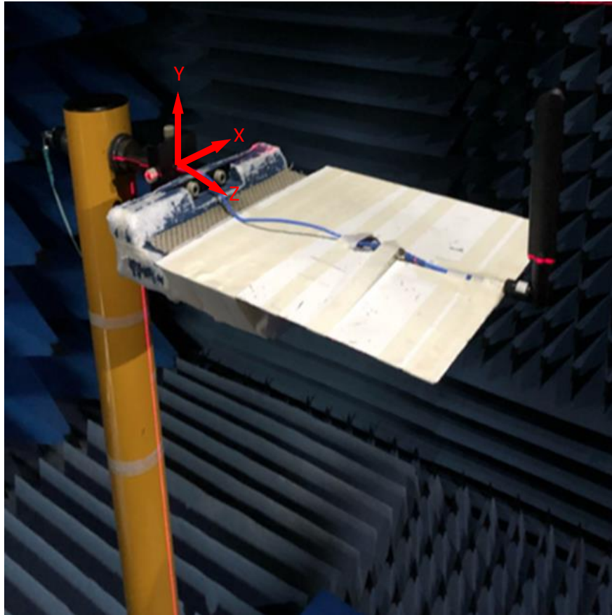
Bent 30x30cm Ground Plane Edge
